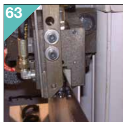
Controllo deviazione lama. Device to check the blade squareness/accuracy.
