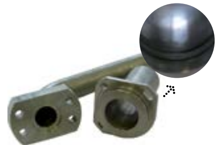
Example of internal seam weld.
