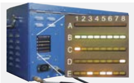
PSS Pro-Service System: Simple functional test with no need to open the unit
