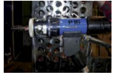
Internal bore welding (I.B.W.)
